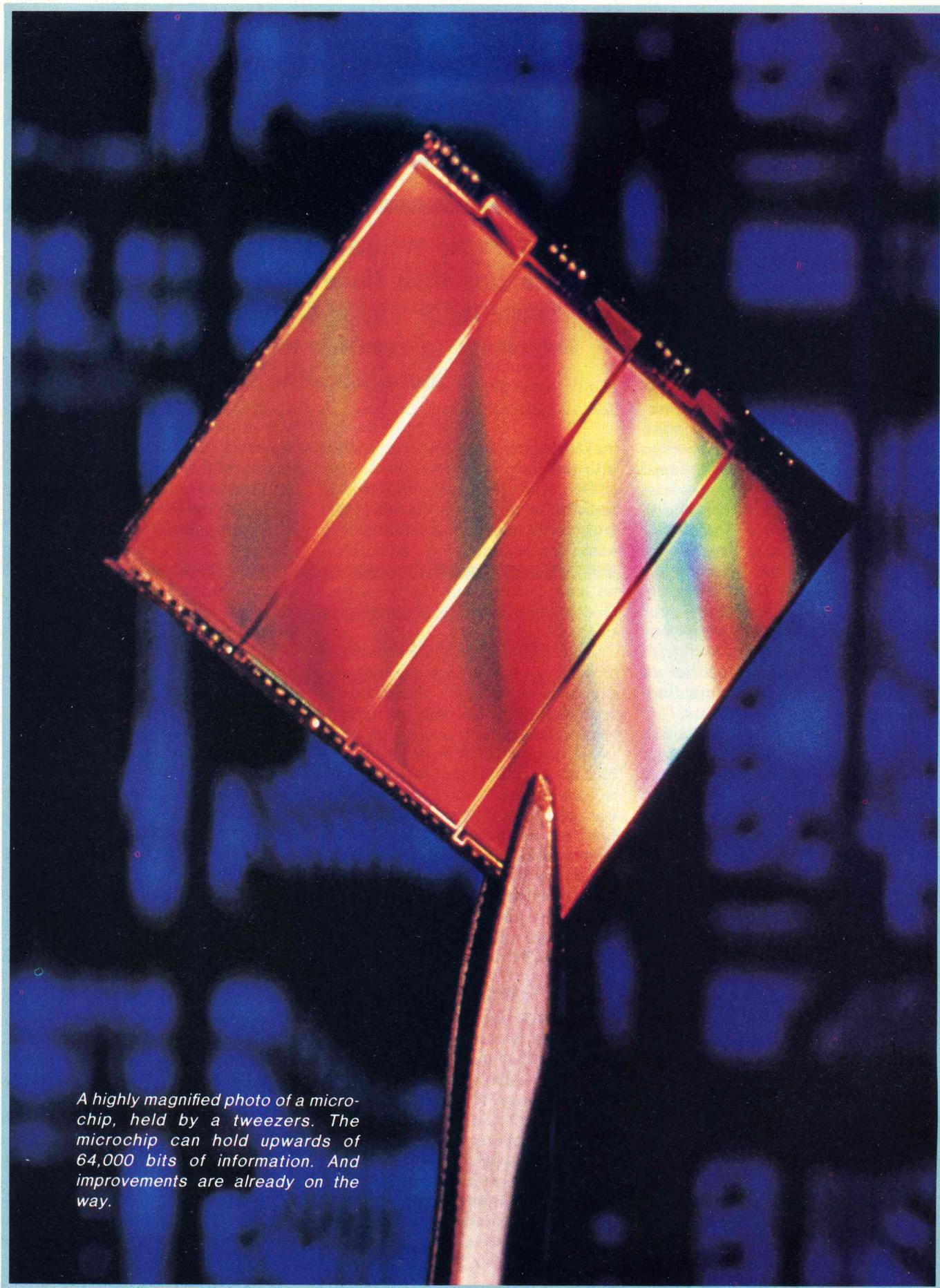
*A highly magnified photo of a microchip, held by a tweezers. The microchip can hold upwards of 64,000 bits of information. And improvements are already on the way.*
